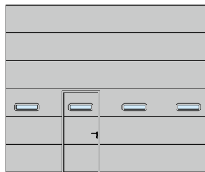
SPU F42, SPU 67 Thermo Panelen met sandwichvensters type D Loopdeurpositie links
